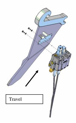
2. Assembly of the control unit with hydrofix:
