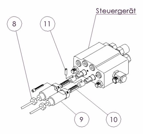
Press adjustable cap **9** against fixing washer **13** and screw on until the lever of the control lever is in control position. Fasten adjustable cap 9 with screw 14 to the control unit. Fasten nut **8**, therefore hold fast the bowden cable cover against rotation. Check, if the bowden cable control works correct and if the control unit regulates correct, when both valve pistons are actuated.
